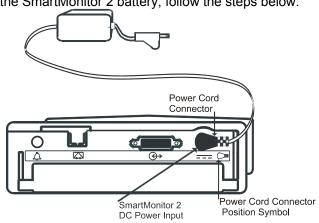
Portable Operation of the SmartMonitor 2
